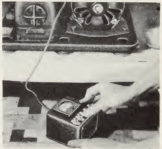
7-41. A capacitor selector unit in operation. (Aerovox Corp.)
